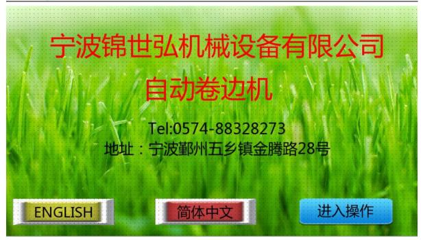
After the machine is powered on, the initial state of the touch screen displays the startup screen, which displays the device name, company address, contact number, Chinese and English buttons in two languages, and the "Enter Operation" button.
